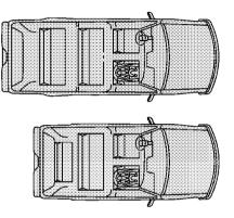
Your vehicle has a right front passenger air bag. A rear seat is a safer place to secure a forward-facing child restraint. See *Where to Put the Restraint on page 1-58.*
